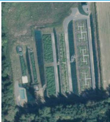
Les Halles treatment plant is designed by Syntea Company to treat domestic wastewater for 800 p.e.. In operation since 2013, the system is composed a French vertical flow system (1<sup>st</sup> and 2<sup>nd</sup> stage) followed by a saturated vertical flow filter and a rough trickling filter, a filtering ditch, and a granulated apatite filter. The particularity of the design is to treat until TN and P only by gravity (no energy on site).
